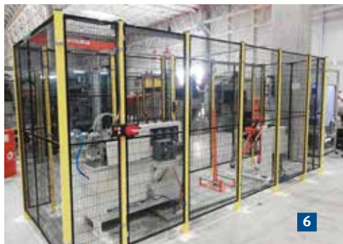
1. Feeding line of coil sheet metal 2. Straightener and Mechanical cutting 3. Sheet Transfer Conveyor 4. Punching process with different tools. 5. Output of finished products 6. Roll forming Line with Fence System
